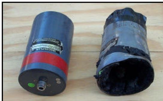
A few months ago the 146.610 repeater went off the air due to a lighting strike to the WROK tower. Being that the tower is a live tower a device called an isocoupler is used to isolate the repeater from the tower. The picture on the left is what a good one looks like, the one on the right is why the repeater was down for about 3 days. Luckily the station engineer for WROK had a spare one laying around so Herb, K9AMJ, was able to replace it at no expense to the club.
