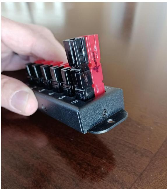
For ham radio and most other applications, the position of the two connectors is very important. This position requires that the PLUS 12 volts be on the right side (red) of the connector when looking INTO the "A", active end.
