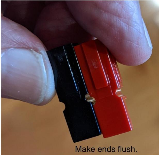
With the shells properly positioned, slide the two shells together until the "A" active ends are FLUSH on the end so the electrical connections will be solid. Because of the tight fit, you may need to gently **tap the back ends** until the front ends are flush.
