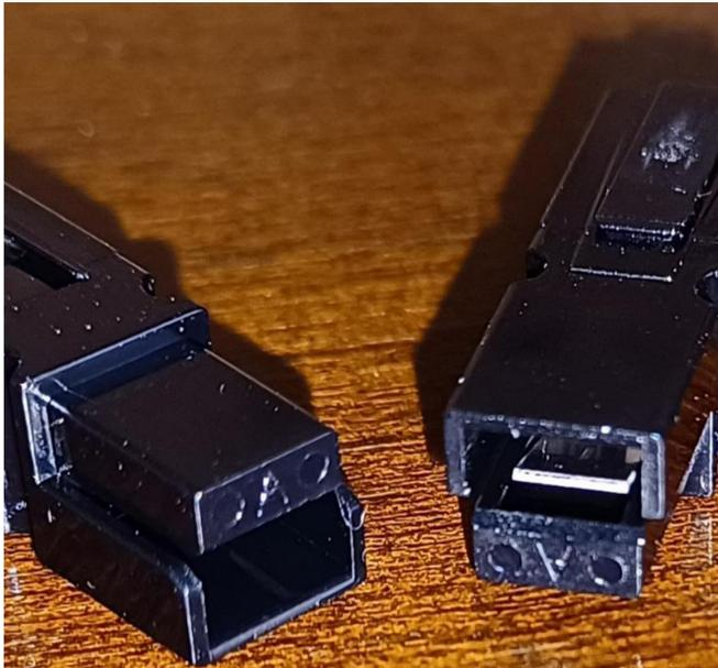
As an example, the embossed "A"s on these two black APs are shown positioned so that either one can be inserted into the other. The "A"s on each AP are in the opposite position so the two connectors can be plugged into one another.
