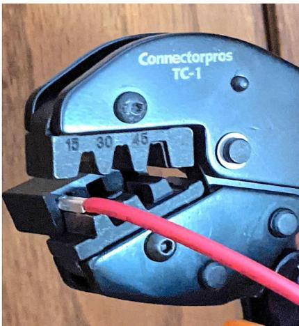
The wire going into the end of this 15 AMP size connector was stripped back 3/8 of an inch.
