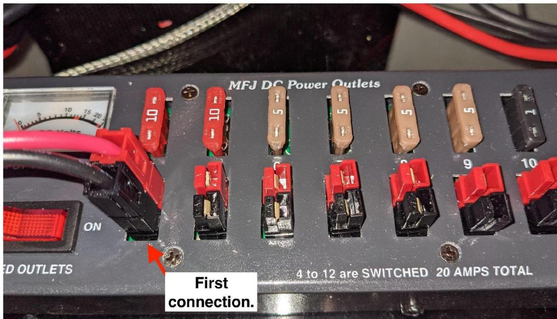
If you are making up Anderson cables for a power strip like that shown above, plug in a pair of empty plastic red and black shells into your power strip initially so that the correct position for the embossed letter "A" is determined before building cables to be inserted.
