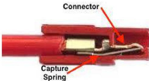
Notice the structure of the built-in "Capture Spring" shown in the cutaway view of the inside of a shell. When inserting a Connector into a shell, be sure both components are flat with no rotation so they can slide over one another properly. As the Connector slides forward the Capture Spring will "click" and the parts will be locked in place. If you do not hear a click, **PULL THE CONNECTOR OUT** and look inside the front to make sure the two parts are level while being assembled.
