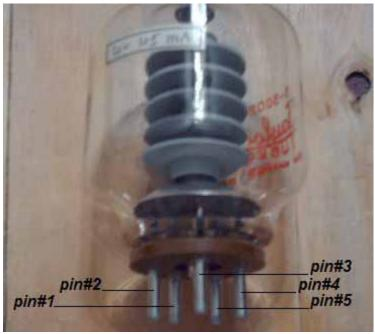
3-500Z tubes are the tubes we usually use in our own Ham Radio Amplifiers. We have always liked them for their power and longevity. Knowing the pin numbers of these tubes are sometimes important especially when your testing the tubes or working on an amplifier that they are installed in.
