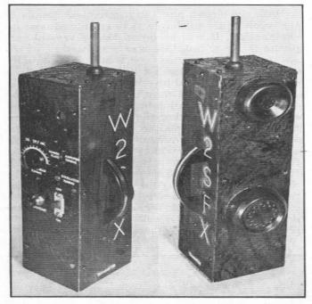
Two views of the 10-meter handie-talkie described by W2SFX. At the left is the control side, showing the receiver tuning, on-off switch, send-receive switch, and the screwdriver adjustments for transmitter tuning. The view at the right shows the side on which the micro-phone and earphone are mounted.
